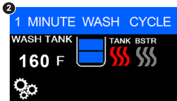
Machine is in normal wash mode
