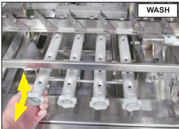
Fig. 63 - Lift and pull forward to remove lower spray arms.
