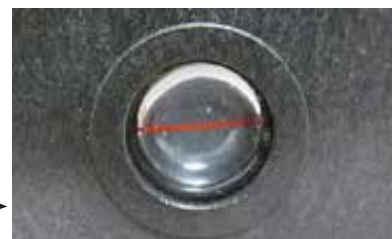
Fig. 77 - Electric valve is closed when red line is horizontal in the valve site window
