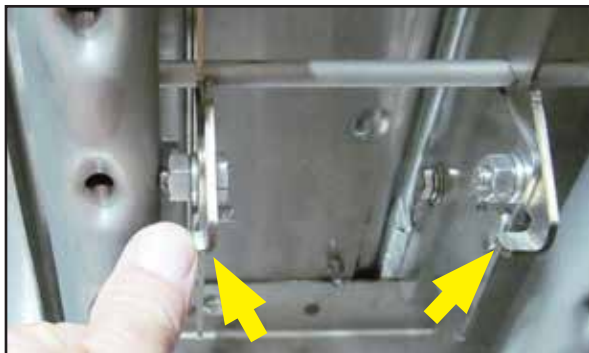
Fig. 64 - Press latches to release upper spray arm.
