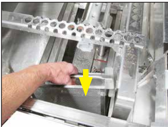
Fig. 84 - Scrap basket and scrap screen
