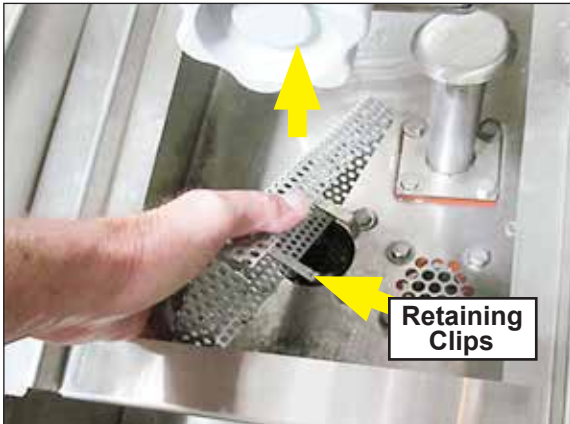
Fig. 83 - Front feed pump suction strainer
