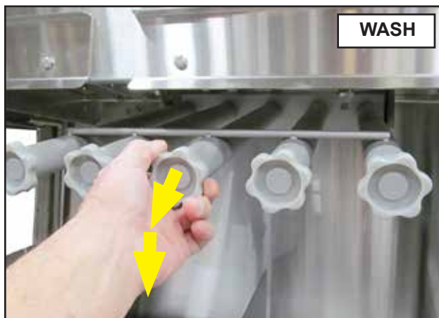
Fig. 65 - Pull forward and down to remove upper spray arms.
