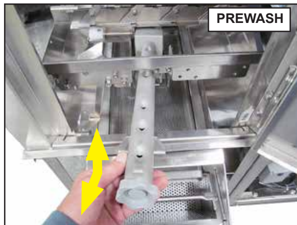
Fig. 63 - Lift and pull forward to remove lower spray arms.
