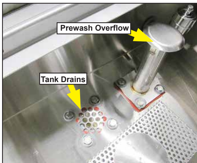
Fig. 72 - Tank drain prewash overflow
