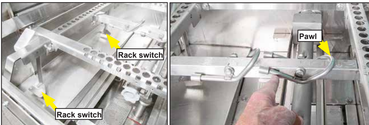
Fig. 79 - Switches and pawls must move freely.
