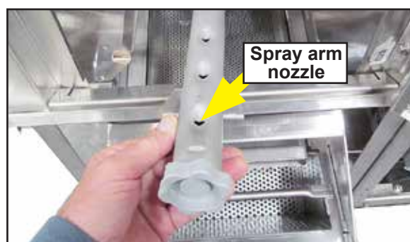
Fig. 68 - Make sure spray arm nozzles are clear.
