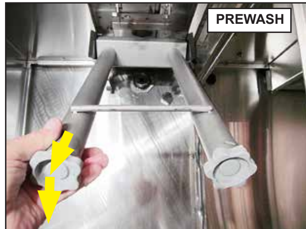
Fig. 65 - Pull forward and down to remove upper spray arms.
