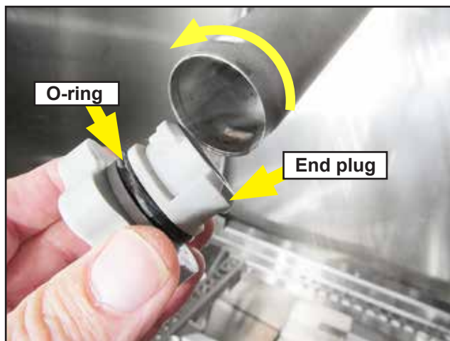
Fig. 66 - Turn plugs 1/4 turn CCW and pull to remove. Check o-rings.
