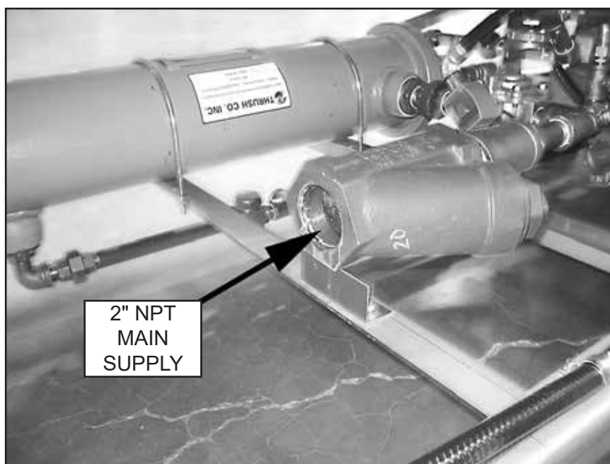
Fig. 27 - Main Steam Supply Line is 2" NPT
