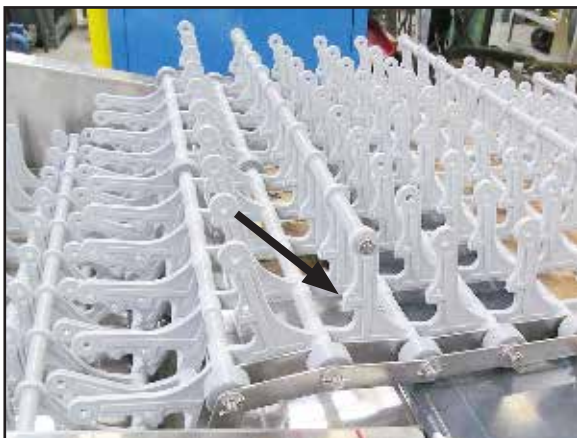
Fig. 5 - Belt peg notches face the load end.
