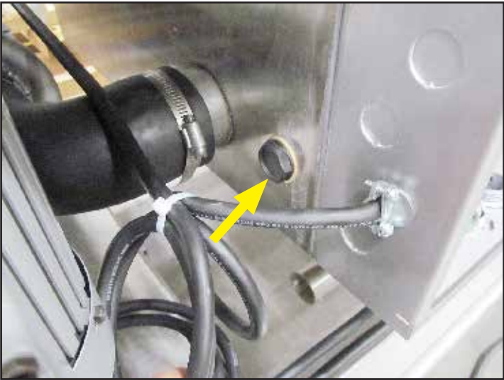
Fig. 31 - Detergent sensor location provided in side of wash tank.
