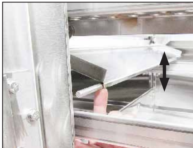
Fig. 9 - Baffles should move freely.
