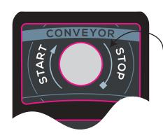
1.The "START/STOP" button is be used to navigate through the menuing system.
