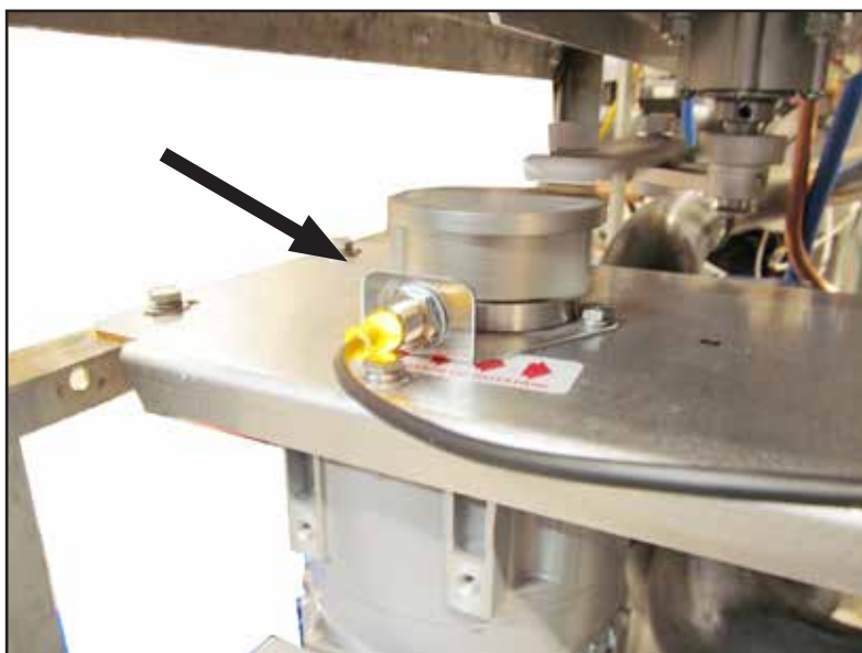
Fig. 30 - Drive assembly sensor
