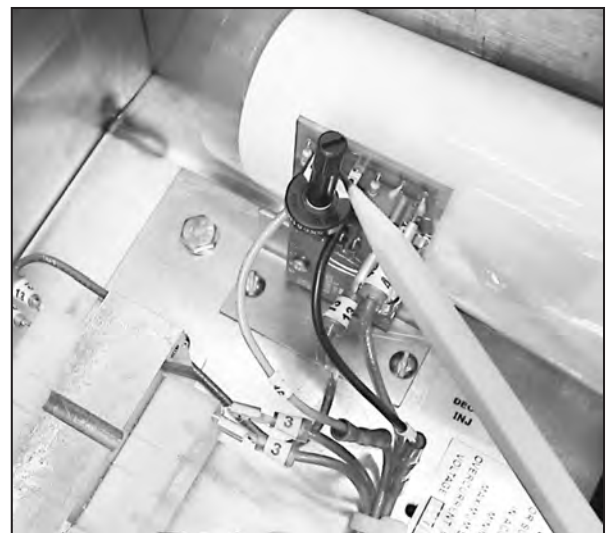
The Deodorizer Injector Speed Control Circuit board is located in the top left corner of the remote control cabinet.
